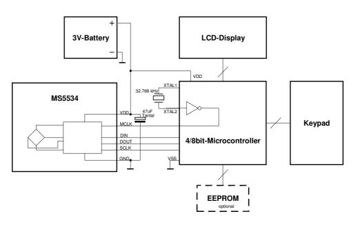
Figure 7: Demonstration of MS5534B in a mobile altimeter.
