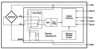
Fig. 1: Block diagram 5534B.
