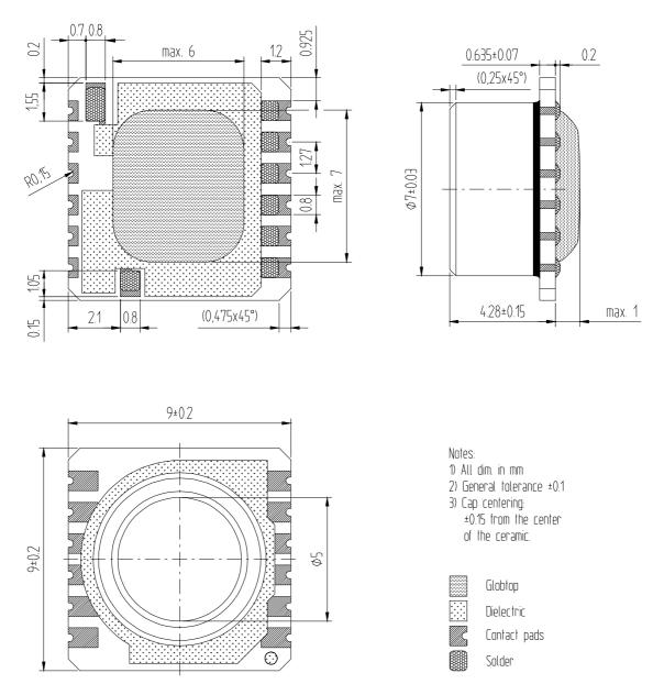
Fig. 9: Device package outlines of MS5534BM.
