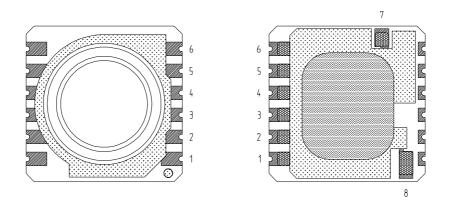
Fig. 2: Pin configuration of MS5534B.
