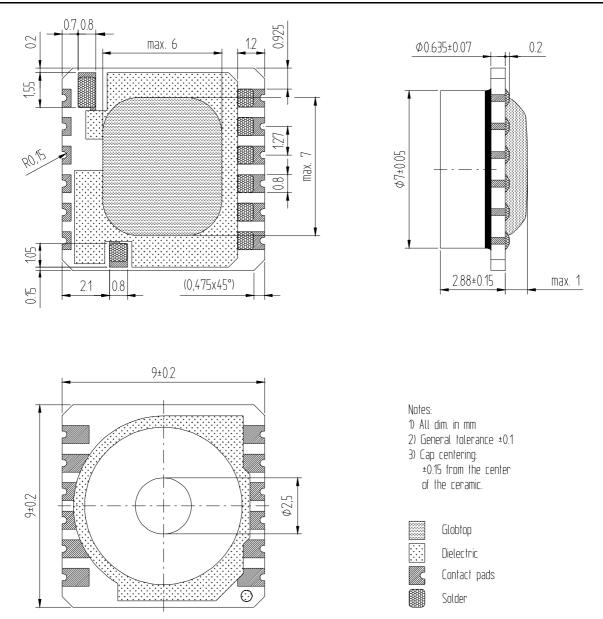
Fig. 8: Device package outlines of MS5534BP.
