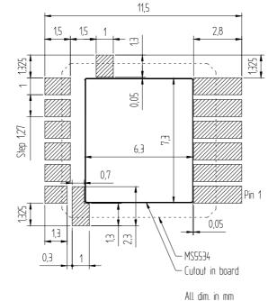
Pad layout for bottom side of MS5534B soldered onto printed circuit board
