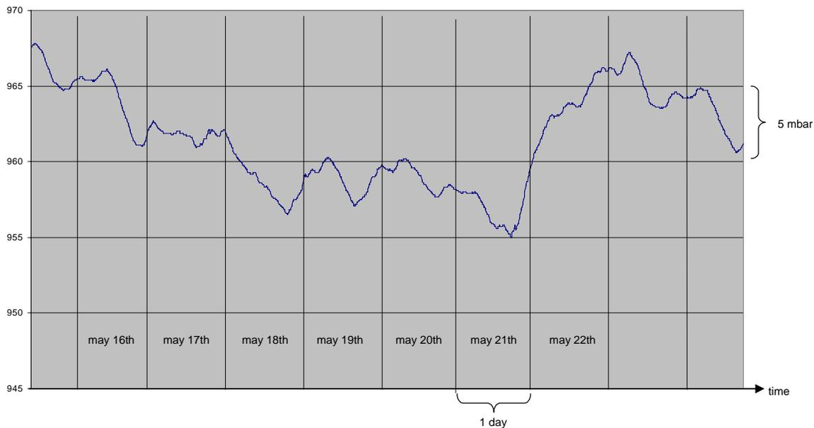
The week started with very sunny and warm weather on Monday 15.5.2000 with a pressure of 967mbar which is around 7 mbar higher than the nominal 960 mbar expected as an average at this altitude. The weather trend during the week was clearly towards bad weather. It can be noticed that during the night the pressure had a tendency to increase which is explained by the fact that the atmosphere cools down increasing the pressure on the ground.
