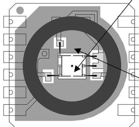
The sensor is protected by a drop of silicone gel. Nevertheless direct water contact might change the sensor properties over time
