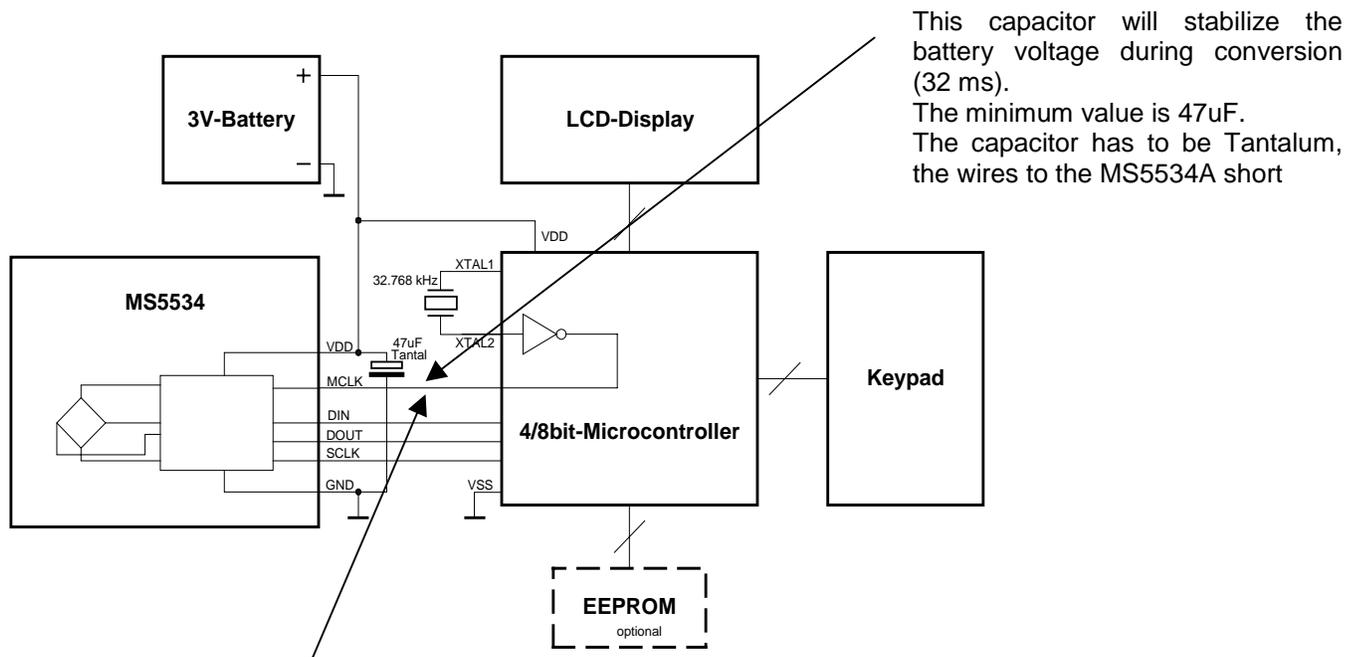
The MCLK signal has to be logic level and jitter free. It is used for the A/D converter and has to be 32768Hz. Higher or lower frequencies will result in noise and increased linearity error of the sensor
