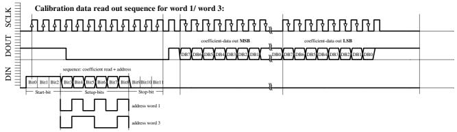
Fig. 6c: W1, W3 READING sequence
