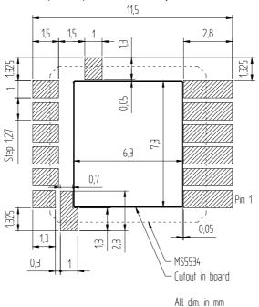
Pad layout for top side of MS5534A (RoHS) soldered onto printed circuit board
