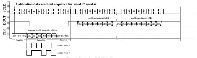
Fig. 6d: W2, W4 READING sequence
