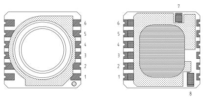
Fig. 2: Pin configuration of MS5534A (RoHS).
