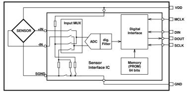
Fig. 1: Block diagram 5534A (RoHS).
